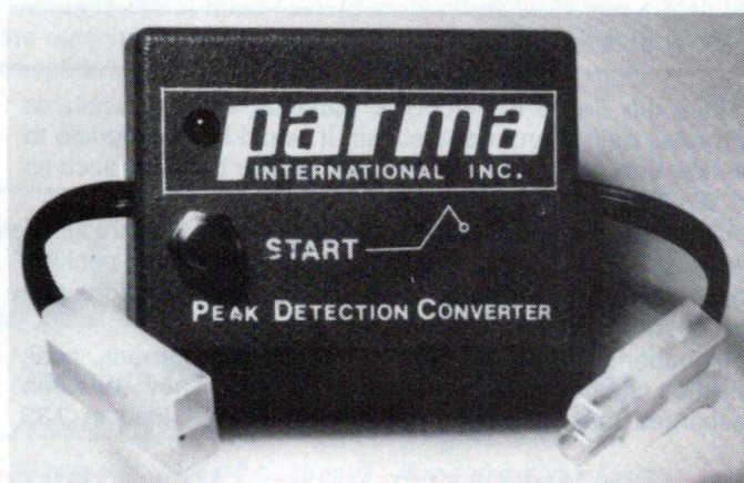
The Parma Peak Detection Converter is a brilliantly simple device that will convert your clockwork timer into a 'Peak Detection Charger' (see diagram below).
